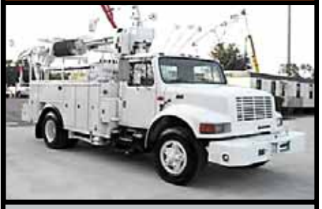
1992 INT 4900, 104,045 Miles, DT466 Turbo Dsl, 195 HP, 5+2 Speed Manual, Hyd Brakes, Tires 10.00R20 90%, Terex 92-42 Commander Style Digger Derrick, 42' Sheave Ht, 3 Stage Telescopic, Behind Cab Center Mount, 2 Outriggers, Upper Ctrl, Capstain Winch, Front Bumper Winch, Stock #4460 $25,900
