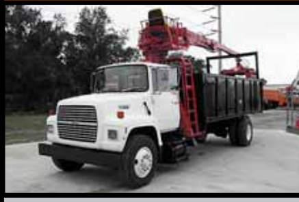
1990 Ford L8000, 132,450 Miles, Ford 7.8L Turbo Dsl, 185 HP, Fuller 6 Speed, Tires 11R22.5 100%, Wheel Base 204", Trash Dump Body 18x4x8, 21.3 Cu. Yd. Cap., 1990 Hood Knuckleboom, 7000# Lower Lift Cap., Behind Cab Mount, Articulated, 2 Outriggers, Stock #4642 $39,900
