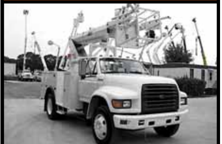
1997 Ford F-Series, 136,441 Miles, 190 HP Cummins Turbo Dsl, Allison MD3060P Automatic, 10R22.5 Tires 70%, Altec AP36 Cable Splicer, 36' WH, 2 Stage Telescopic Boom, Center Over Axle Mount, 1 Man Basket, 500# Capacity, Stock #6139 $29,900
